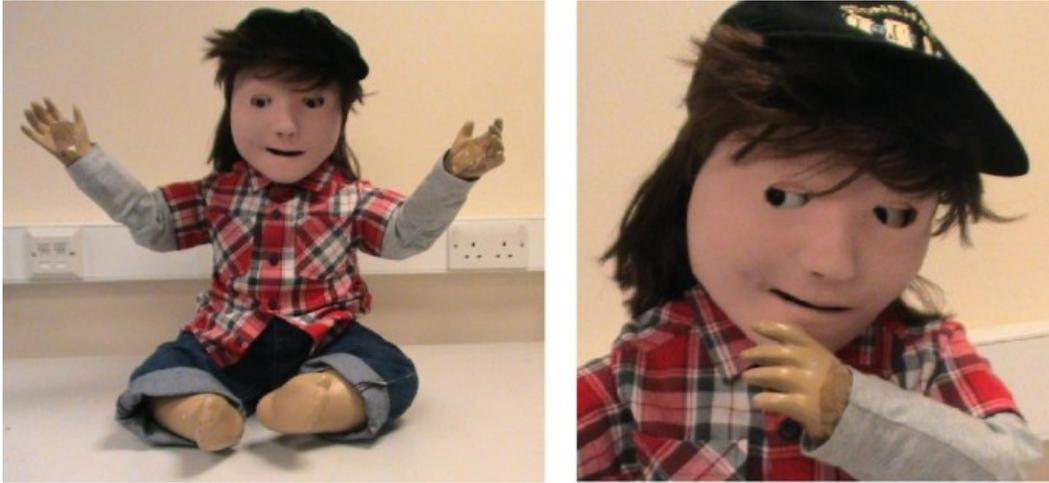
Figure 3.7: KASPAR 1b, the second and improved model of minimally-expressive robots built by the University of Hertfordshire [Robins et al., 2010]
