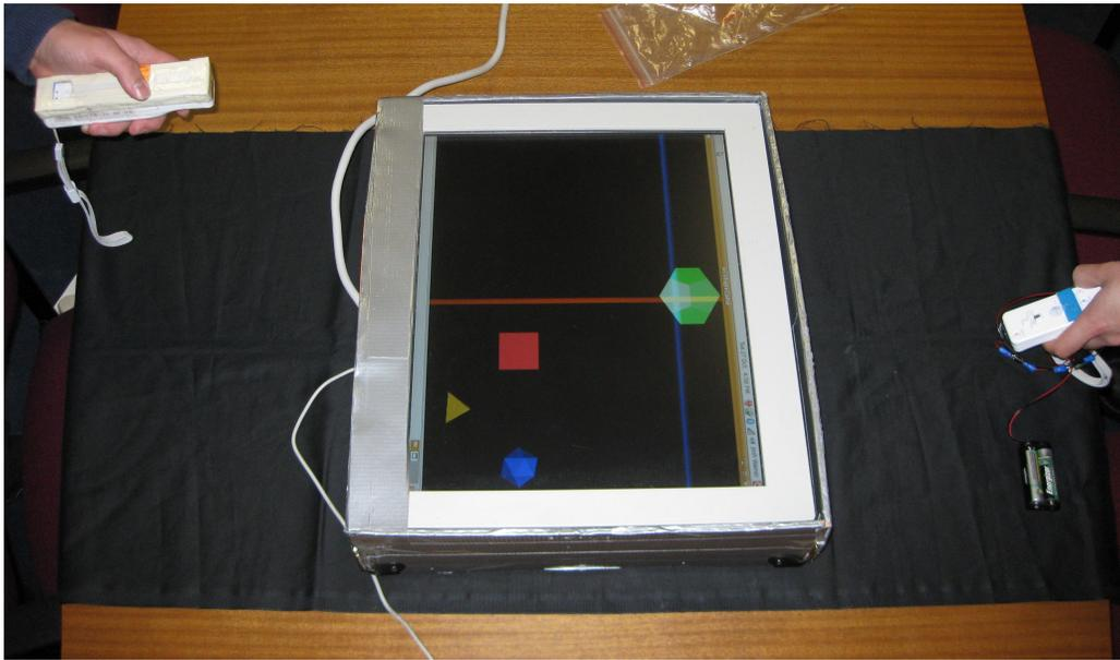
Figure 4.4: The setup for playing “Tilt and roll”. The player on the left (stand-in for the child with autism) controls the location of the orange selection line, while the player on the right (stand-in for the human adult or the humanoid robot) controls the location of the blue selection line.
