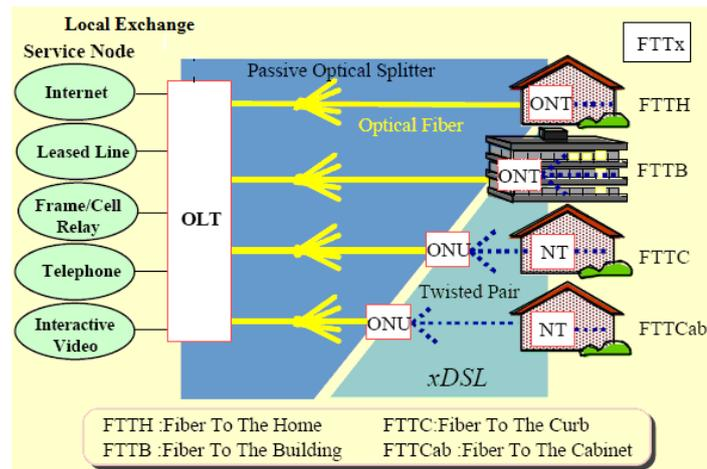
**Figure 1-2 Fibre-to-the-x architectures [12]**
